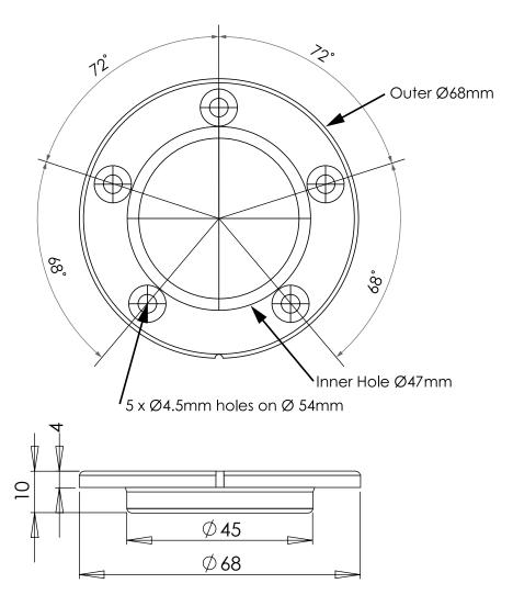
The mounting diagram shows the mounting hole and central hole locations and sizes.
