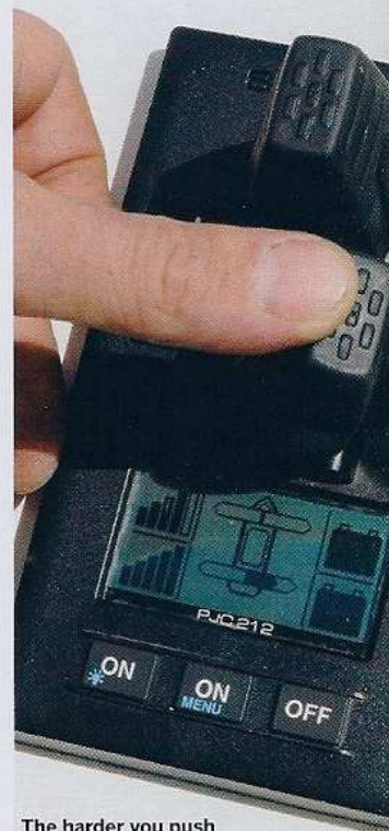
The harder you push the paddle switch the more thrust you apply
