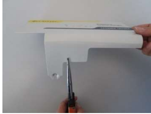
Break out the metal tongue with flat-nose pliers
