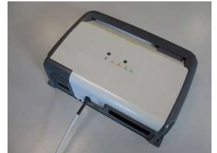
Break out the metal tongue with flat-nose pliers
