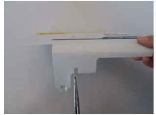
Break out the metal tongue with flat-nose pliers
