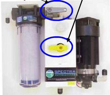
Valves in flush position
