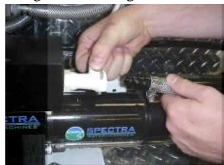
Connecting brine discharge hose to Clark Pump
