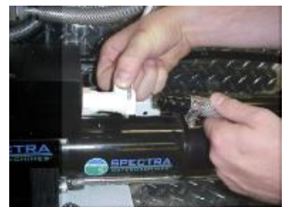
Connecting the Brine Discharge service hose. 11
