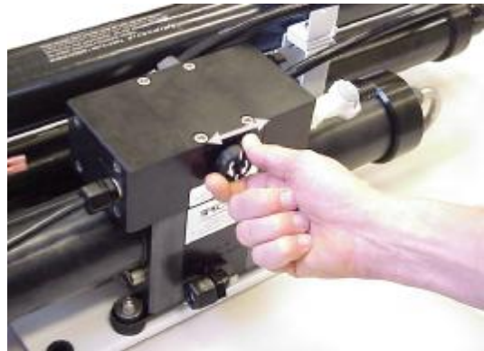
Connecting brine discharge hose to Clark Pump
