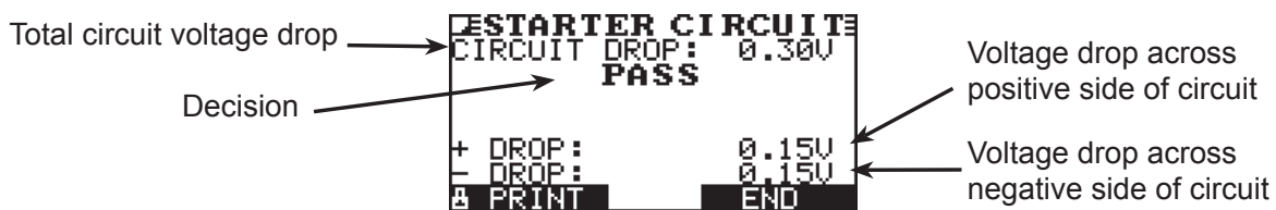
Figure 19: Starter Circuit PASS Result
