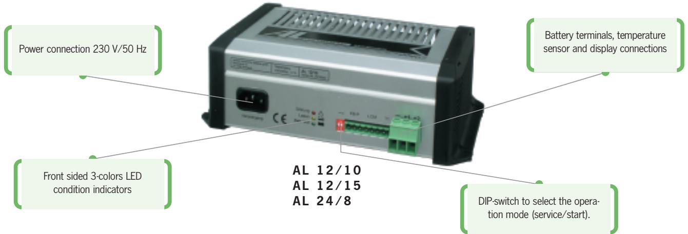
The charger AL 12/15 FI was designed especially for small installations. It is based on the technique of automatic charger AL and combined with shore power connector. This reduces the installation procedure, as only the
