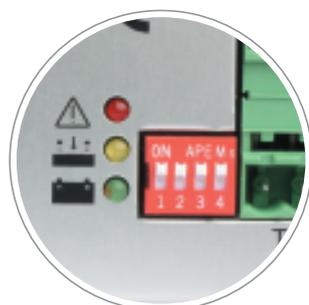
**Adjustment on different battery systems.**
