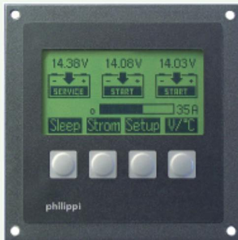
The charging monitor indicates the voltages of the attached groups of batteries also without shore power connection. During the charging operation it indicates additionally all relevant charging parameters, like charging current, temperatures of the batteries and the device status. Also the charging current can be reduced, the configuration changed, and the SLEEP mode activated.
