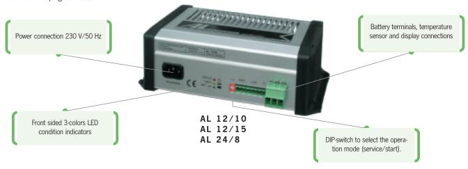
The charger AL 12/15 FI was designed especially for small installations. It is based on the technique of automatic charger AL and combined with shore power connector. This reduces the installation procedure, as only the unit and a shore power connector is needed. The RCB/MCB device and the socket are in the front side. Another connection in the back output enables the safe connection of further consumers 230 V/50 Hz.
