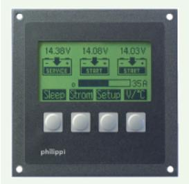
The charging monitor indicates the voltages of the attached groups of batteries also without shore power connection. During the charging operation it indicates additionally all relevant charging parameters, like charging current, temperatures of the batteries and the device status. Also the charging current can be reduced, the configuration changed, and the SLEEP mode activated.
