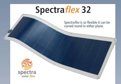
The Spectraflex is a solar panel made from a spectrum splitting amorphous silicon cell design that converts very low levels of light to useable solar energy. Unlike other types of amorphous silicon technology the Spectraflex is very stable over many years where others degrade rapidly soon after deployment. Bypass diodes are connected across each cell so the panel is also shadow tolerant.
