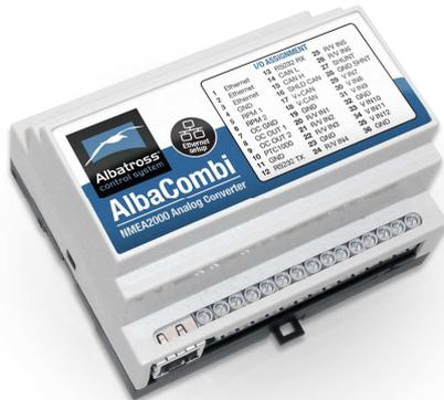
The Alba-Combi is a state of the art analogue to NMEA2000 converter that covers the most demanding applications. The Alba-Combi has six 0V to 32V channels and another additional six channels can be configured in voltage or resistive 0 to 600 ohms mode. There are also two RPM inputs available, one PTC and one shunt input.
